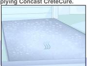
2. Spray or brush an even layer of Concast CreteCure on the concrete surface.
